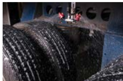
Each truck contains a disinfecting unit that sprays the wheels upon entering and when exiting the farm.
